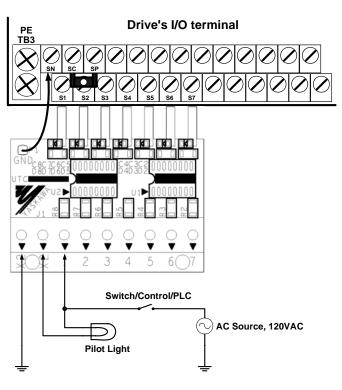
One channel shown as example, remaining channels are identical.
